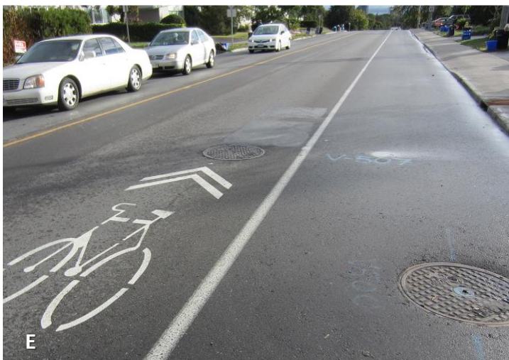
A: Worn sharrow on Beechwood (credit: Vanier Cycles) B: Snow-covered sharrow on Laurier (credit: Brian Smith) C: Sharrow eliminated by road patching on Beechwood (credit: Vanier Cycles) D: Sharrow in a legal parking space on Byron (credit: Lana Stewart) E: Sharrow confounding safe and/or legal cycling lane position on Meadowlands. Empty parking lane, with blacked-out sharrow in the dooring zone, re-painted but still in the dooring zone and too far right for a narrow travel lane (credit: Heather Shearer). F: Sharrow placed in contravention of Book 18 (speed limit) on Carling at the 417 (credit: Heather Shearer)
